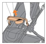
Locate the unlock buttons on each arm of the snack tray. Press the buttons and pull the snack tray away from the stroller.
