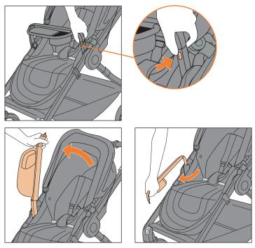
Press the swivel release button and pull the tray upward. The tray can swing up and swivel out of the way to make it easier to get your child in and out of the stroller. For safety, tray should be fully re-attached or fully removed before folding.
