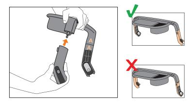
Align the arms in the correct orientation as shown above. Make sure the letters "A" and "B" on the tray match with the corresponding arms. Insert the metal rod on the tray into the top of the arm until you hear a "CLICK".
